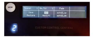
Scene **Save** or **Restore** take place after you turn the leftmost knob to display a scene number, and press the respective button below that knob. The **Save** or **Restore** action are immediate; no confirmation is asked for.
