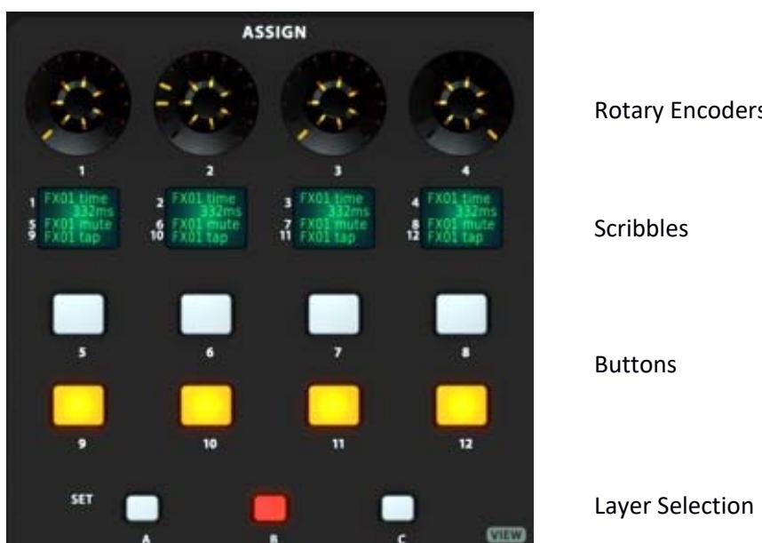
A series of 3 buttons at the bottom of the section enables selecting one of 3 layers of user controls layers [A, B and C]. When addressing user controls to get or set data, the layer name and encoder or button number must be provided. A small LCD displays the functions the rotary encoders or buttons are assigned to.
